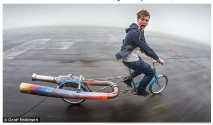
Remodelled: Colin Furze took four months to build hid bike extending it at the back to protect riders from the heat generated by the jets but still extremely close to the gas canister holding the fuel
